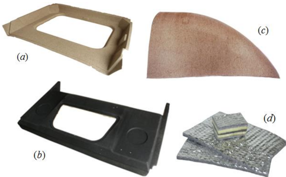
Figure 2. Product examples of interior components made from developed sound-absorbing composites: ceiling elements of the tractor "Belarus" (a, b); cover of the inner wheel arches of the tractor "Belarus" (c); multilayer noise-reducing structure for the cab of railway locomotives (d)
